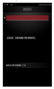
7. If a USB drive is connected with a new version of the Always Up Display software, version, the display will give the option to perform the update:
