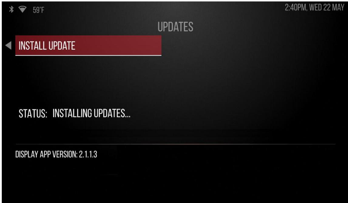
9. Once the update is loaded, the red notice “UPDATE COMPLETE, CYCLE KEY” will appear. Turn the ignition key to OFF and then back to IGN to restart the display. You’re done!
