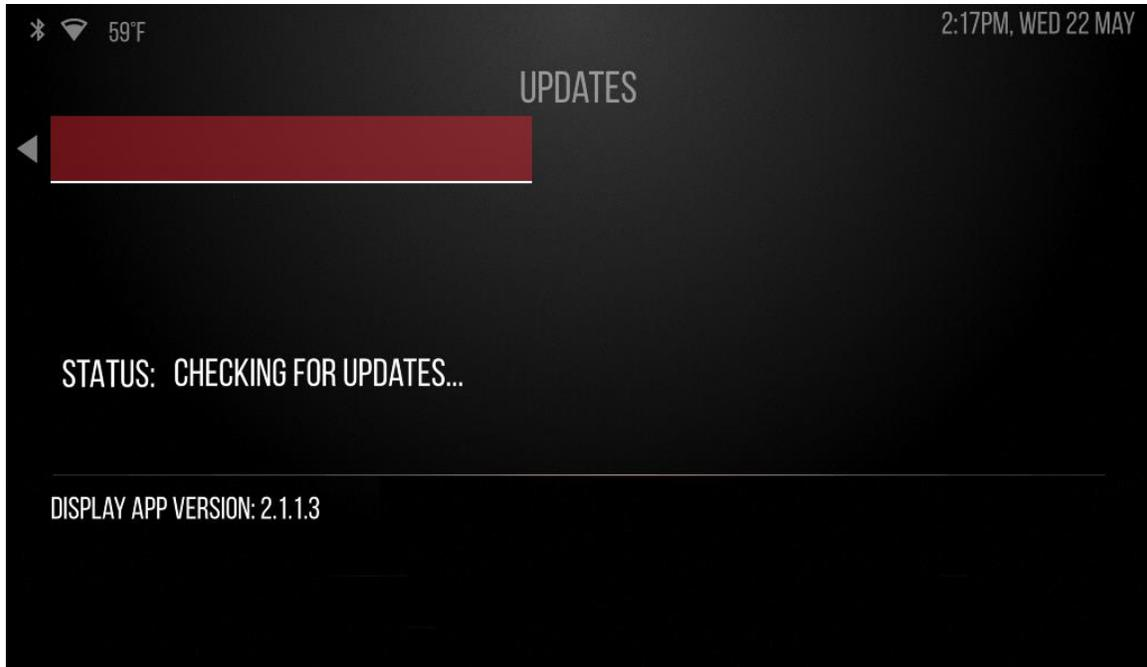
7. If a USB drive is connected with a new version of the Always Up Display software, version, the display will give the option to perform the update:
