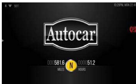
NO DISTRACTION MODE reduces distractions by only populating gauges as required
