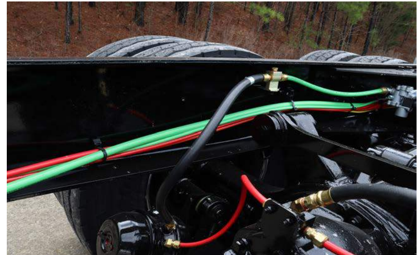
COLOR-CODED AIRLINES airlines are color-coded for ease of fault finding
