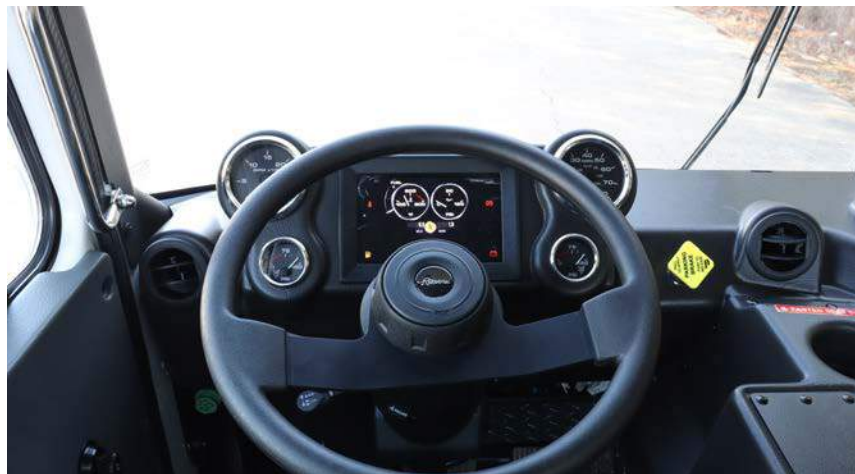
FOCUS MODE only displays gauges and key information
