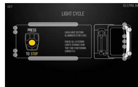
LIGHT CYCLE TEST driver can check all lights with automated light sequence
